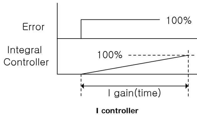
**7) WEB\_34 PIDGain RAMP : PID Gain Ramp Time Setting**
