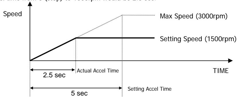
**Setting example 2** If FUN\_33 is set to 'Ref Speed' and speed command and acceleration time is set to 1500rpm and 5 seconds, respectively, it takes 5 seconds to accelerate from the standstill to 1500rpm.
