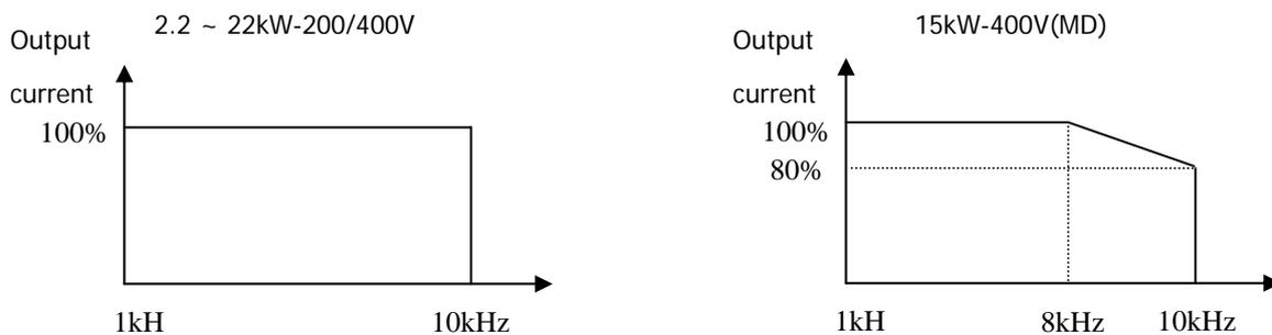
② The above graph is only applied when the inverter is operated in the allowable temperature. Pay attention to the air cooling when the inverter is installed in a panel box, and the inside temperature should be within an allowable temperature range.
