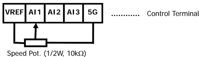
4.8.3 Adjusting Ai1 Gain and Bias (example of analog input Ai1 setting)
