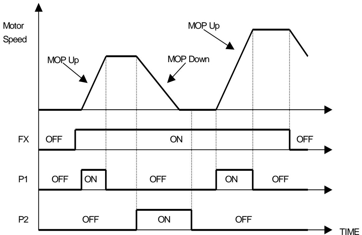
(MOP Save example 2) In case terminal input assigned to MOP Save function is ON, operation speed at that instant is memorized and operates at the saved speed when operation resumes.
