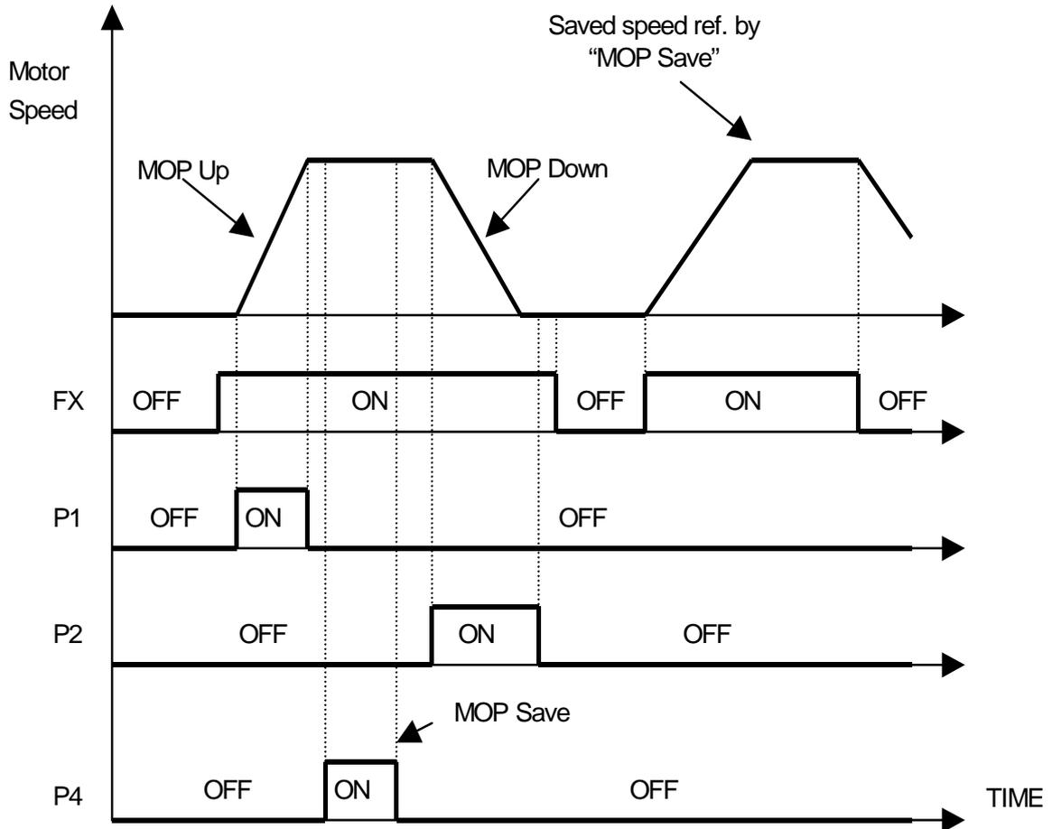
(MOP Clear setting example 3) To clear the saved speed by MOP Save function, use "MOP Clear ON/OFF". If MOP Clear is ON during running, the inverter decelerates its speed to zero speed. If MOP is ON during stop, this function resets the speed reference to "0".
