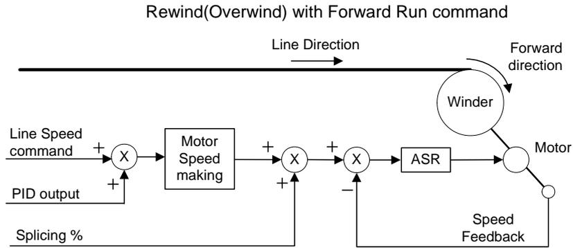
Figure 1. Roll Rotating Direction at the time of Rewind/Overwind Setting, Forward Direction Operation Command
